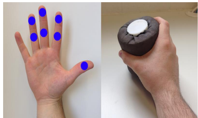
Figure 4 Positions of conductive foam sensors relative to the hand while grasping the HandLog
