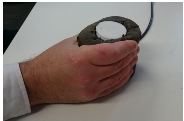
Figure 6 The vertical grip: whole hand squeeze of the HandLog for the HeliGrasp game
