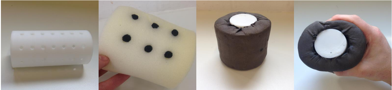
Figure 1 HandLog components and usage (from left): 3D printed core; foam sleeve (white) with embedded conductive foam (black) sensors; HandLog device with core and sleeve; Whole hand finger flexion gesture
